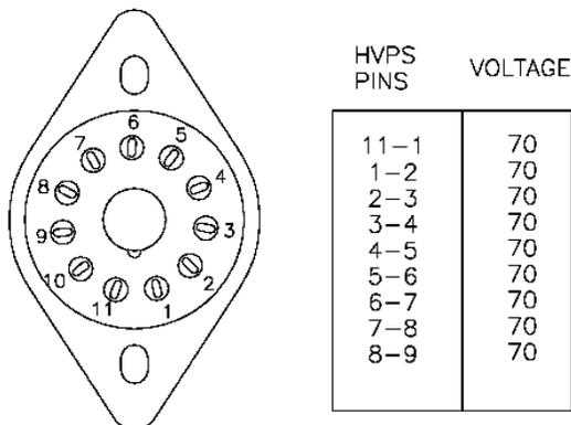
10. Turn off the instrument power, and reconnect the PMT tube, and then reassemble the sensor, including desiccant bag replacement per the Maintenance Schedule requirements (Section 5.1).
