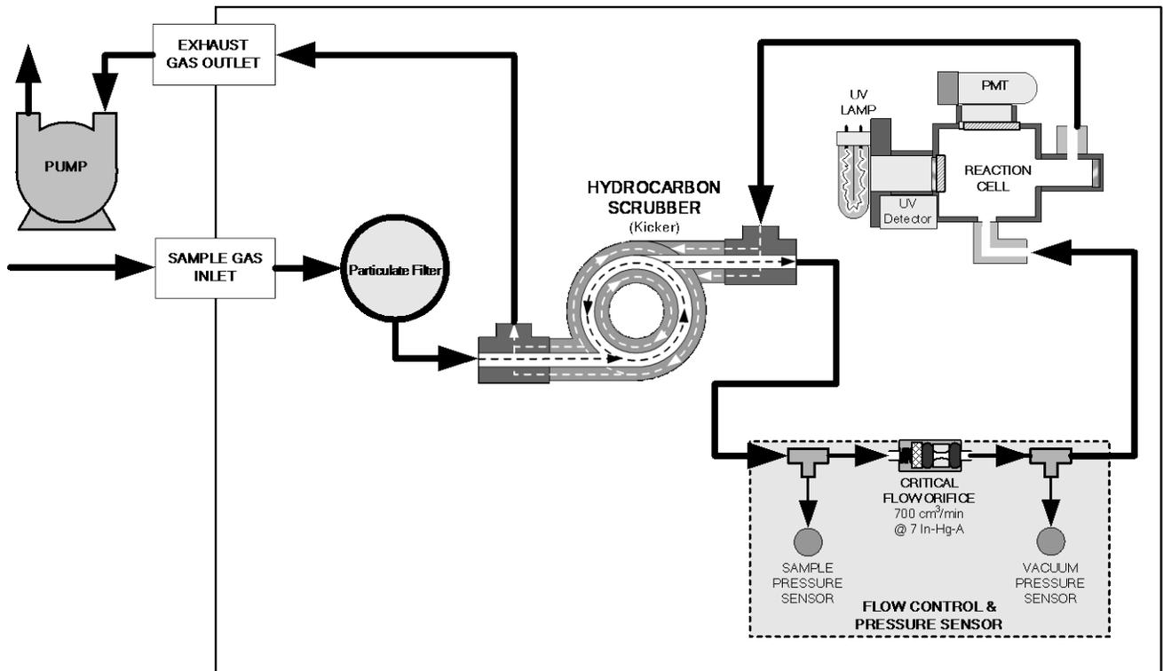
Figure 2-22. N100H Pneumatic Flow with Hydrocarbon Kicker Option
