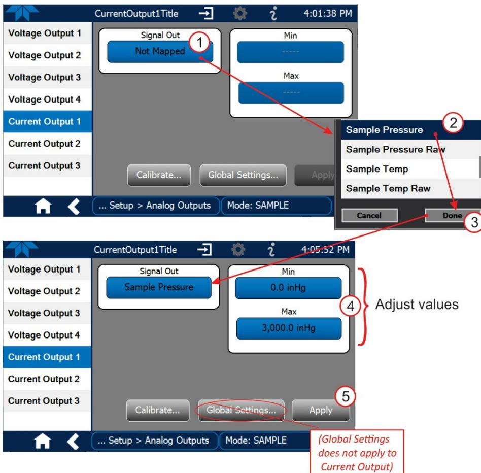
**Figure 2-47. Analog Output Configuration for Current Output, Example**
