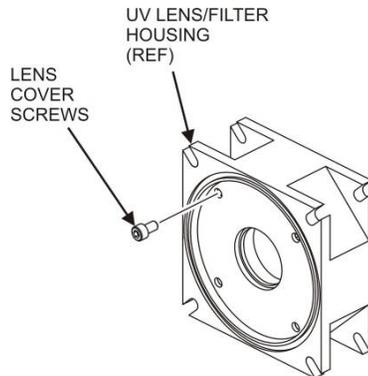
**Figure 5-28. UV Lens Housing / Filter Housing**
