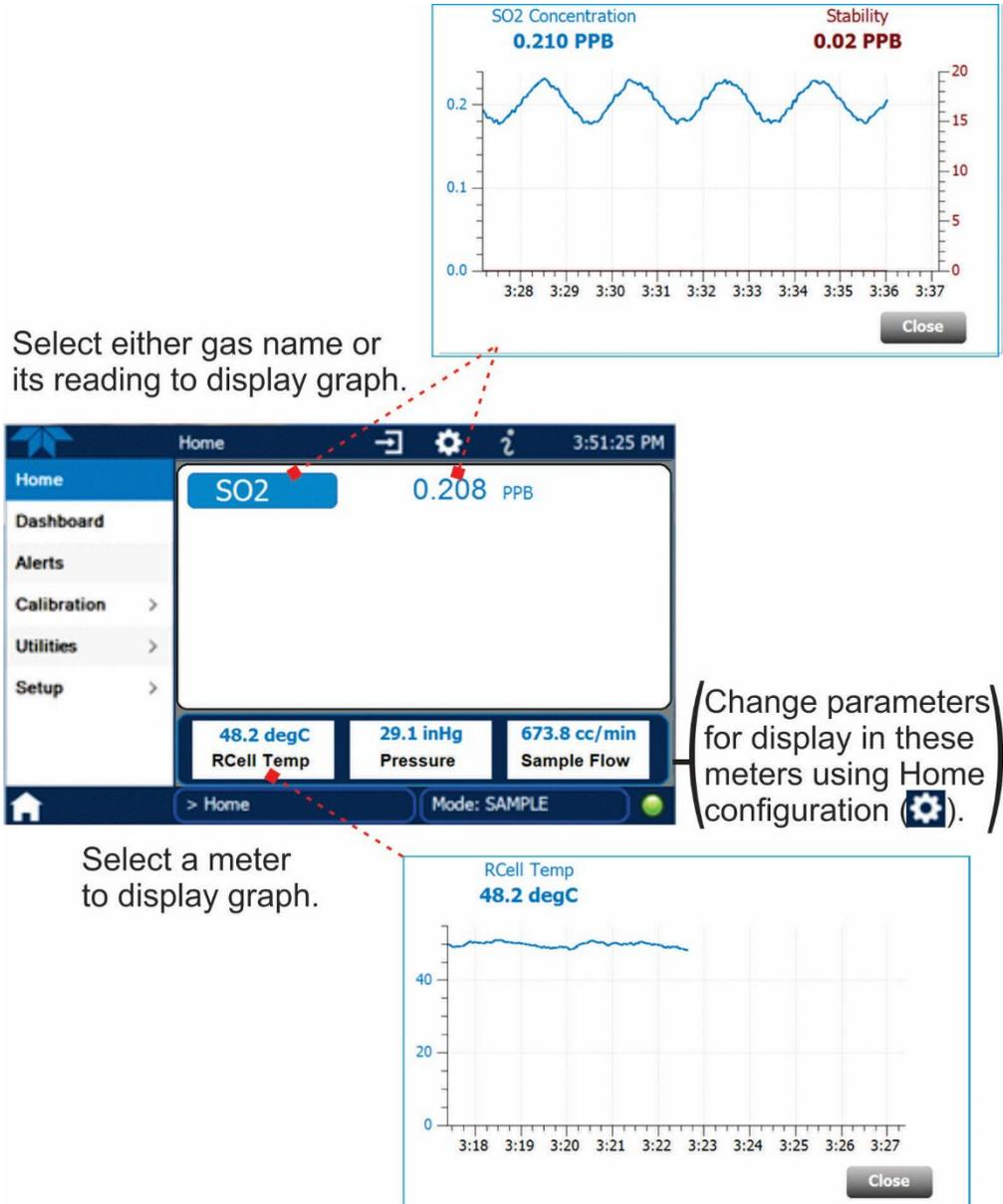
Figure 2-28. Concentration and Stability Graph (top) and Meter Graph (bottom)
