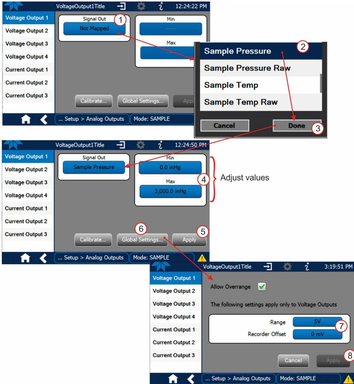
**Figure 2-46. Analog Output Configuration for Voltage Output, Example**
