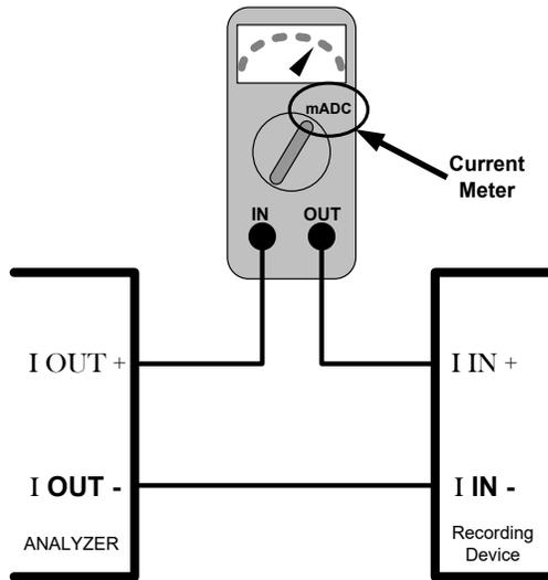
Figure 2-50. Setup for Checking / Calibration Current Output Signal Levels
