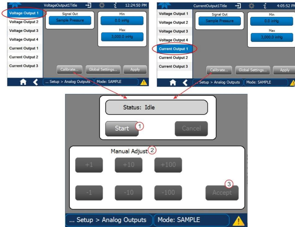
**Figure 2-48. Analog Output Calibration, Voltage or Current**
