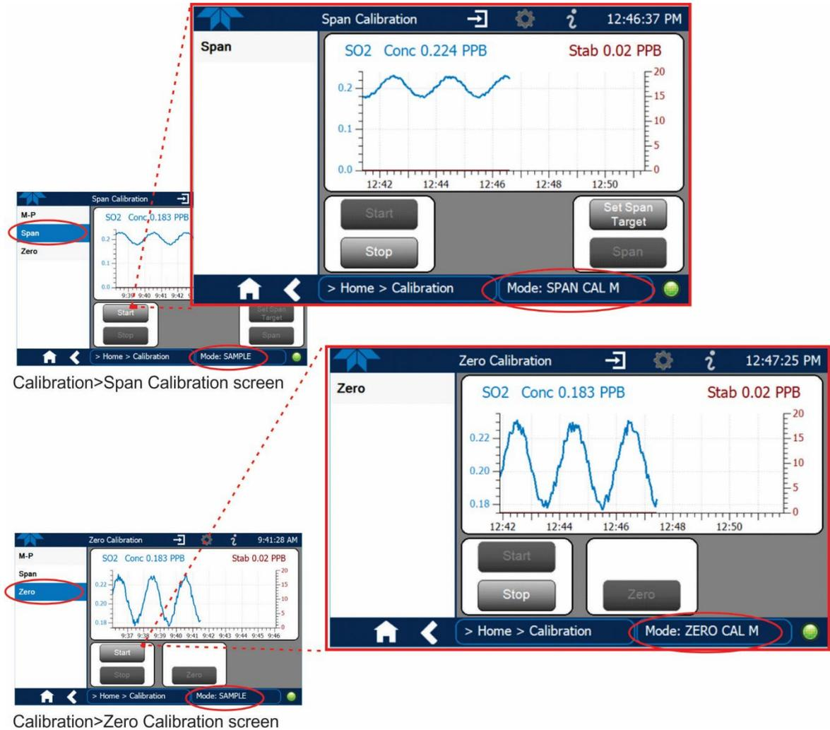
**Figure 4-4. Zero and Span Calibration Screens**
