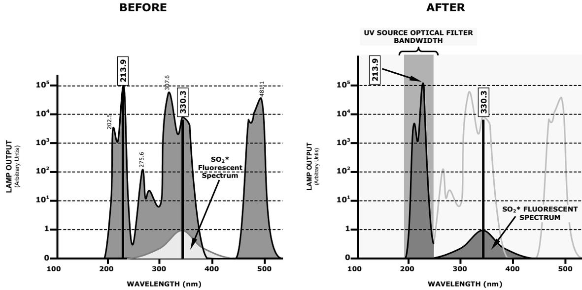
Figure 6-5. Excitation Lamp UV Spectrum Before/After Filtration
