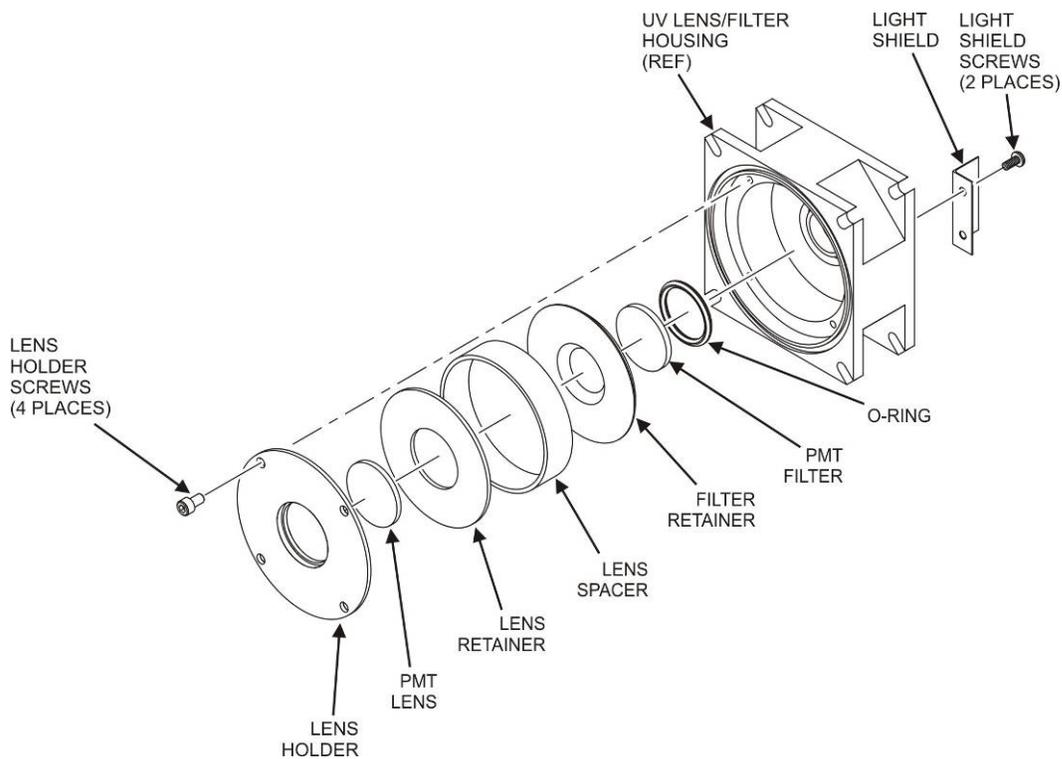
**Figure 5-29. PMT UV Filter Housing Disassembled**
