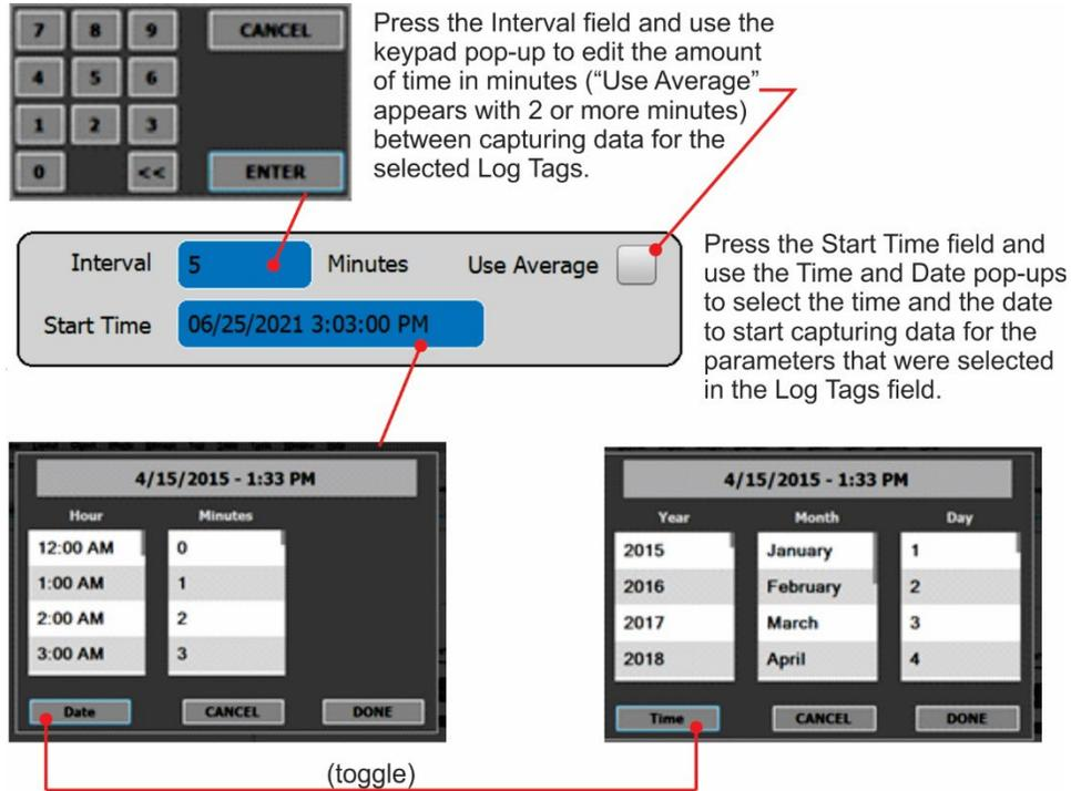
Figure 2-36. Datalog Periodic Trigger Configuration
