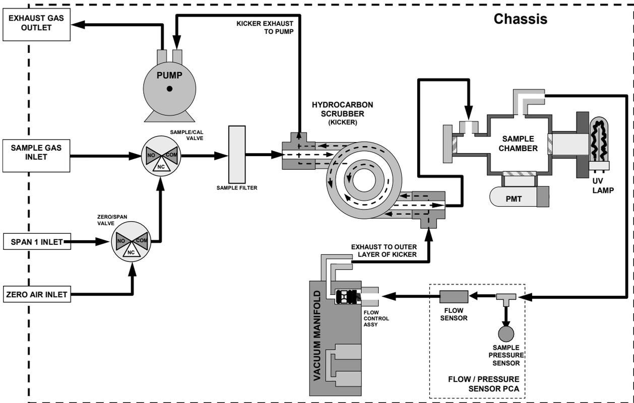
Figure 2-17. N100 Pneumatic Flow with Zero/Span Valves Option
