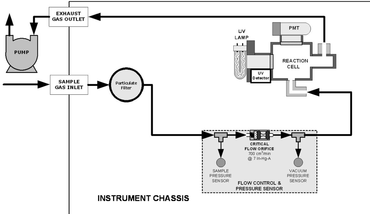
Figure 2-16. N100H Pneumatic Flow Path
