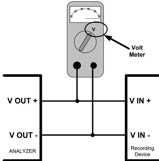
Figure 2-49. Setup for Checking / Calibrating DCV Analog Output Signal Levels
