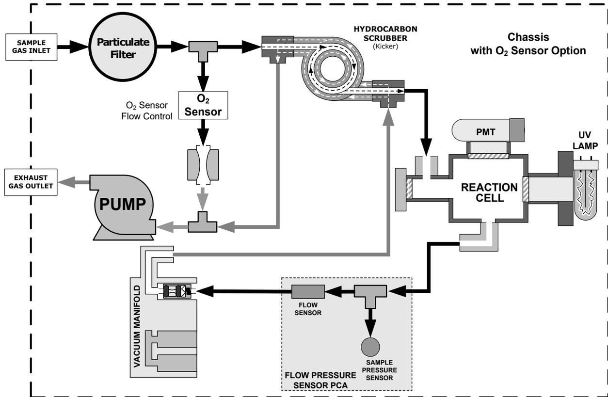
Figure 2-20. Pneumatics with O<sub>2</sub> Sensor
