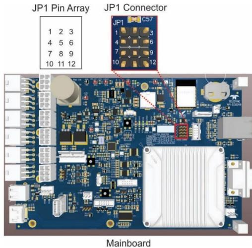
**Figure 2-7. Mainboard JP1 Location and Pin Arrangements**
