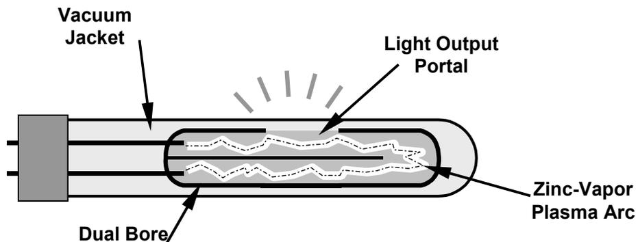
Figure 6-4. Source UV Lamp Construction
