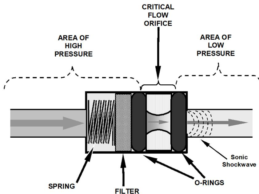
**Figure 6-9. Flow Control Assembly & Critical Flow Orifice**
