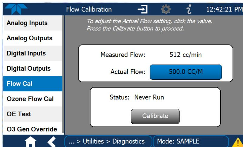
Figure 5-8. Flow Calibration Menu
