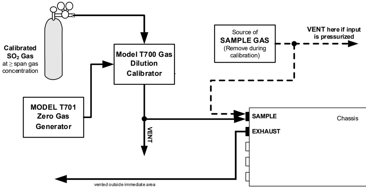
Figure 2-8. N100 Basic Connections from Gas Dilution Calibrator
