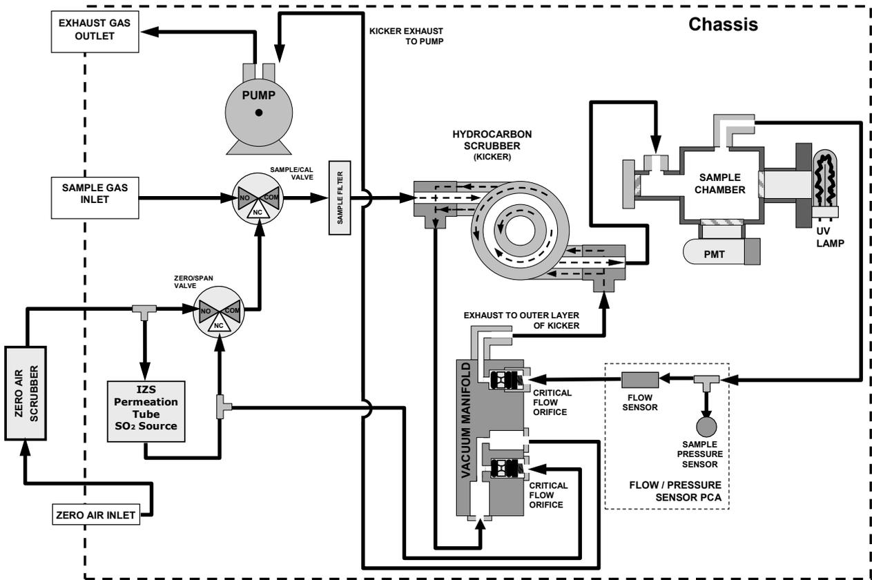
Figure 2-19. N100 Pneumatics with IZS Option
