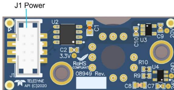
**Figure 5-18. UV Detector Board Connector**
