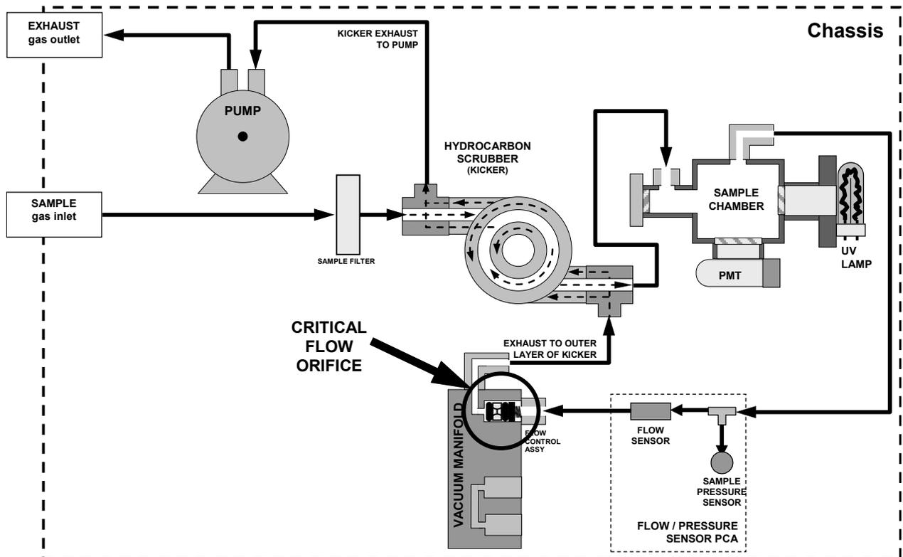
Figure 6-8. Gas Flow and Location of Critical Flow Orifice
