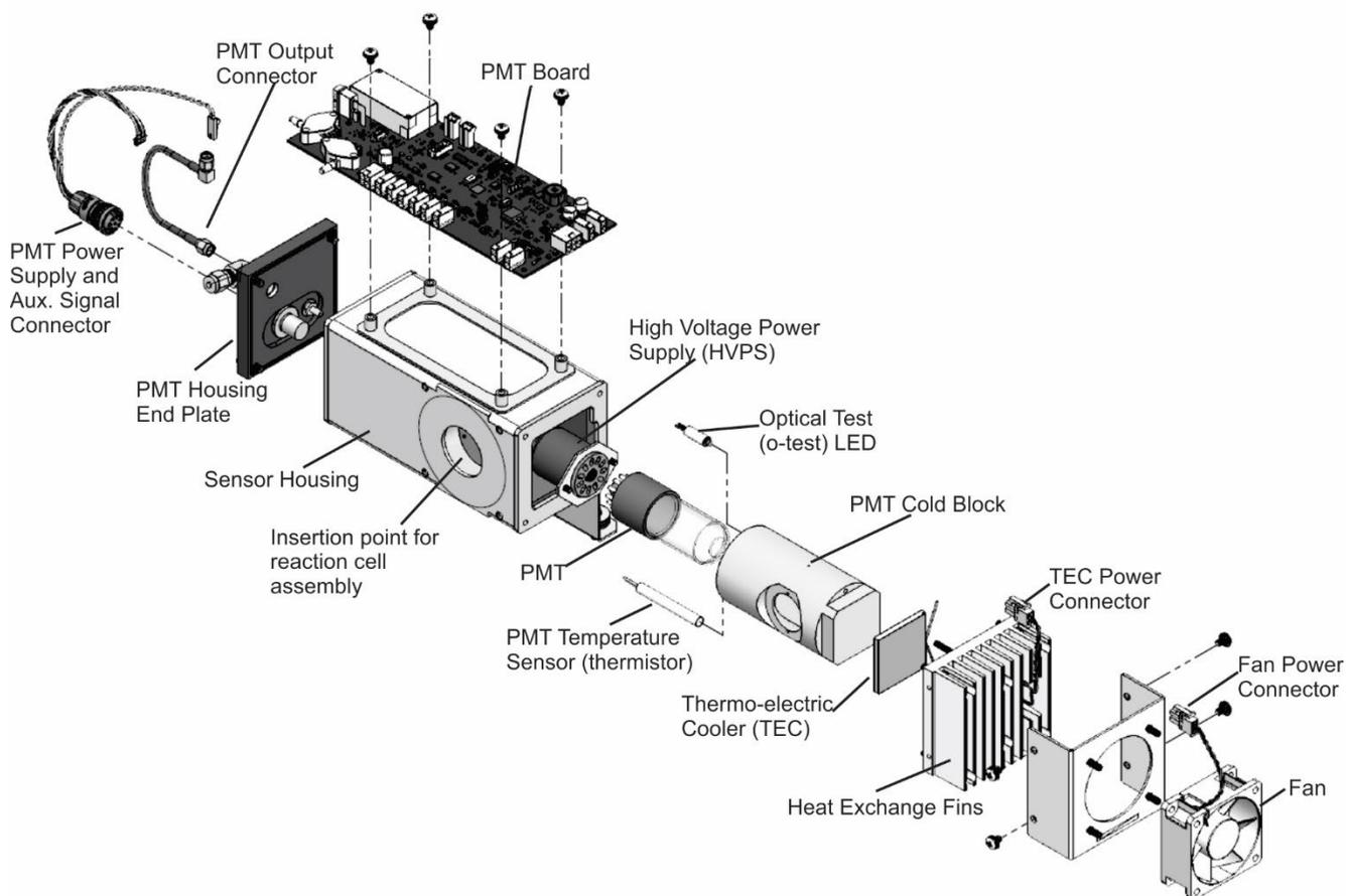
**Figure 5-33. Sensor Assembly**
