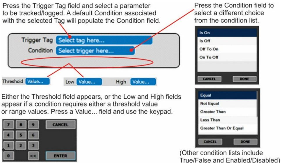
Figure 2-37. Datalog - Conditional Trigger Configuration
