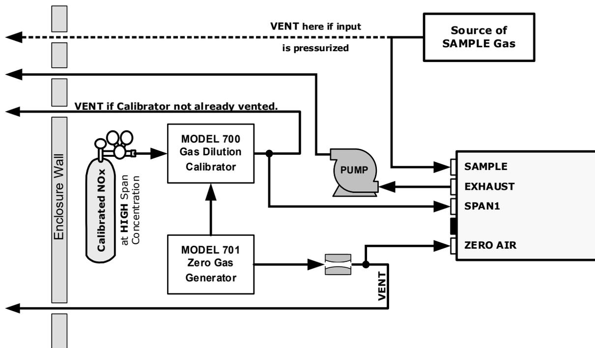
Figure 2-11. Gas Line Connections with Z/S Valves Option
