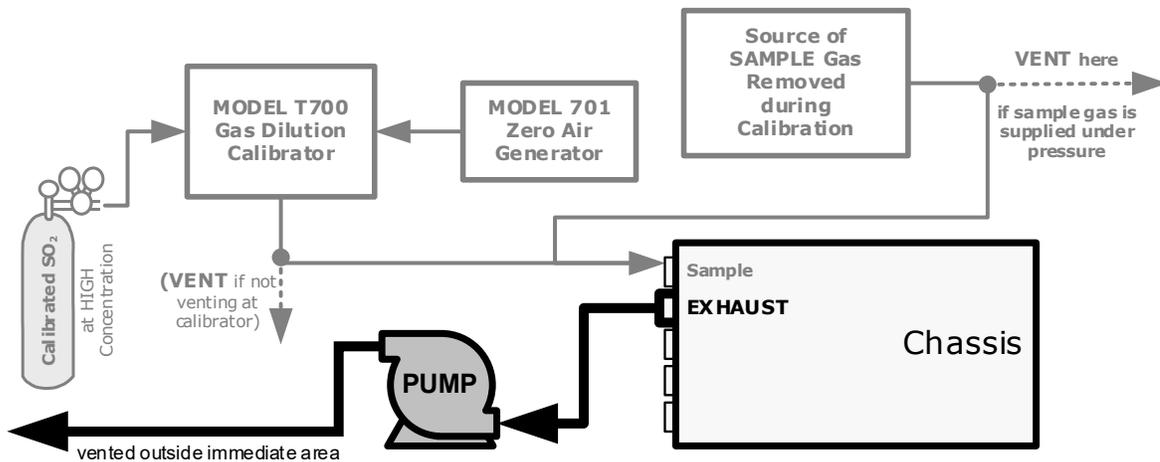
Figure 2-9. N100H Basic Connections from Gas Dilution Calibrator
