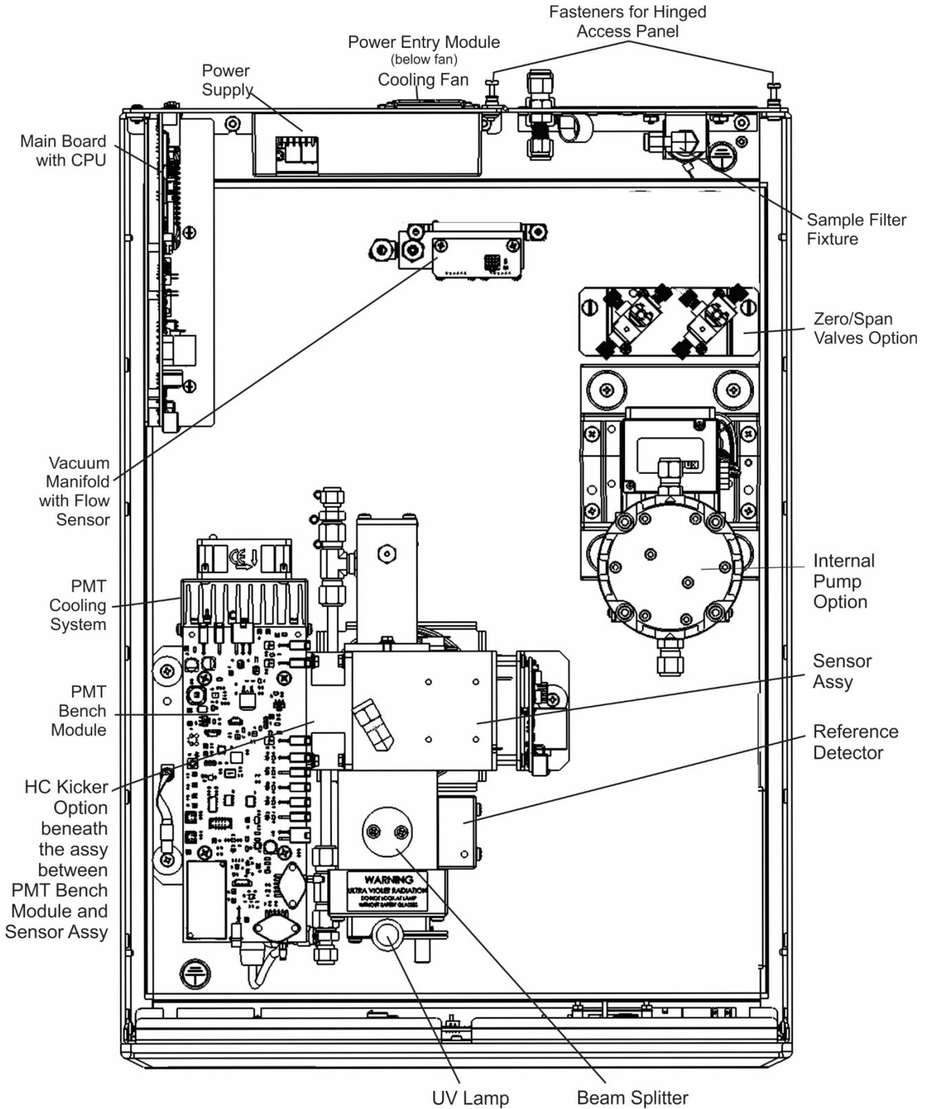
**Figure 2-4. N100H Internal Chassis Layout**
