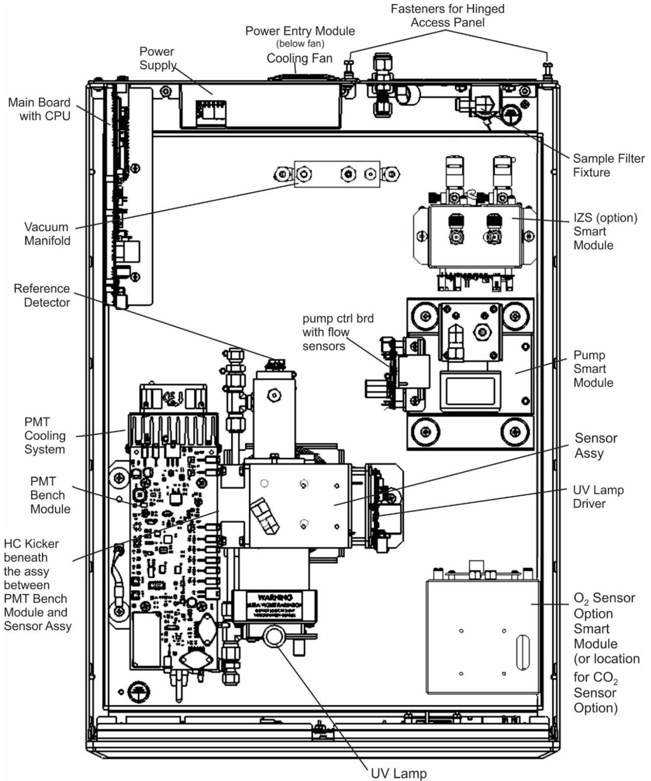
Figure 2-3. N100 Internal Chassis Layout
