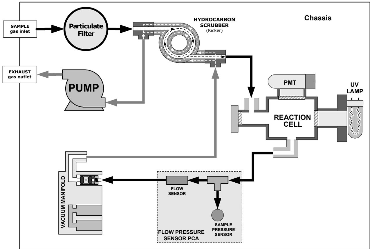
Figure 2-15. N100 Pneumatic Flow Path, Basic Configuration
