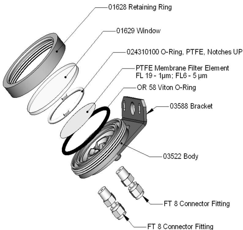
**Figure 5-5. Replacing the Particulate Filter**
