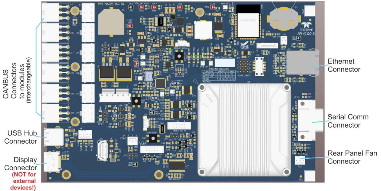
Figure 5-23. Mainboard Connectors
